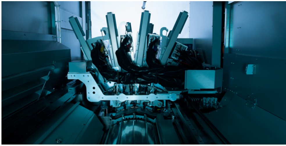
SAMBA™ modular printheads are the powerful heart of the Jet Press 720S.
