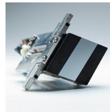
Samba printhead used in the Jet Press 750S. Invisible to the naked eye, 2048 nozzles are contained in the silver coloured silicon chip that measures just 44 mm wide by 18 mm deep.
